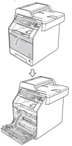
2 Hold the green handle of the drum unit. Pull the drum unit out until it stops.
